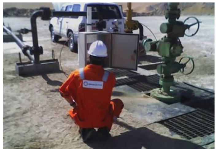
SensorNet Data Engineer performing a drive-by data service on a water injection well
